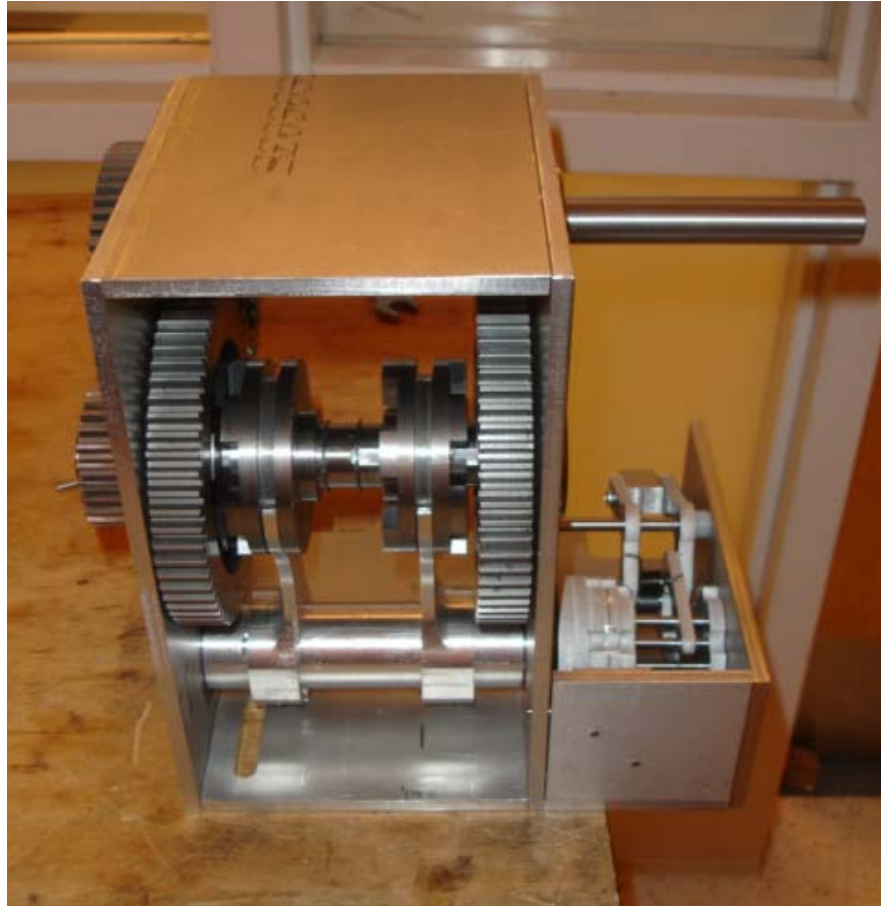
Figure 24: Photograph of the gate 2 prototype. This prototype demonstrated the capability of a complex actuation system with a more complete representation of a baja gearbox. We successfully demonstrated a system to prevent meshing issues.
