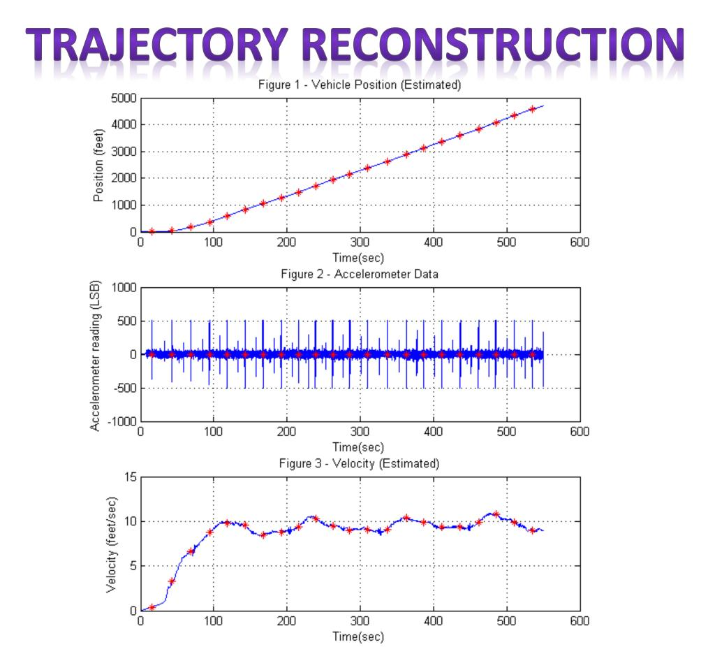
The Kalman filter calculates how strongly it should trust a measurement. By knowing the variance of the measurement and the estimate, the Kalman filter weights the past estimate and the data from the sensor to obtain the best estimate possible. Measurements become more accurate with more measurements
